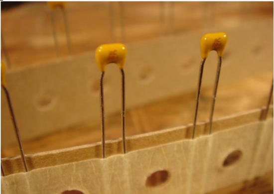
There are several values of ceramic capacitors in WTPA2. Most are 0.1uF – there are lots of them. 0.1uF caps are common on many boards – they are often used for power supply filtering (we call it bypassing). The two 20pFs are used to stabilize the crystal oscillator. Ceramic caps are never polar as far as I know.
