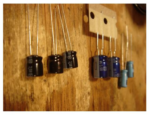
Electrolytic caps look like this. The colors aren't important, the numbers are. They'll all be labeled. The big guys are the main power supply filters, the 22uFs are filters for analog references and also the audio output AC coupling, and the 1.0uF caps are inter-stage audio coupling caps.
