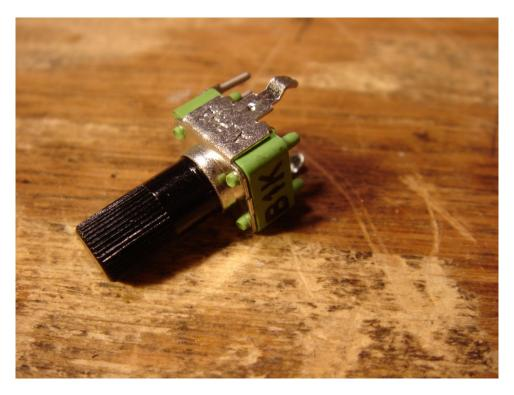
Potentiometers are often called pots. These are variable resistors which internally wipe copper leaf over a carbon strip. They let us adjust electrical parameters by changing the a resistance ratio inside the component. **THERE ARE 2 KINDS OF POTS IN WTPA2** but physically they look very similar! You've got to read the text to tell them apart.
