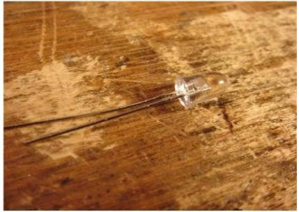
The LONG LEAD on the LED is the anode (positive). It is oriented towards the top of the PCB everywhere in WTPA. There is also a flat on the other side of the LED (the cathode) which matches the diagram on the PCB.
