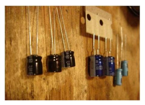
There are three kinds of electrolytic caps: the 470uFs (the big guys), the 22uFs (the black ones) and the 1.0uF (light blue in this photo). The colors aren't important, the numbers are. They'll all be labeled. The big guys are the main power supply filters, the 22uFs are filters for analog references and also the audio output AC coupling, and the 1.0uF caps are inter-stage audio coupling caps.
