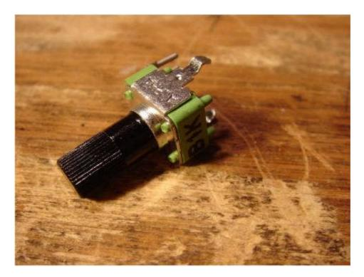
We can see that this pot says B1K (not to be confused with B2K). This means it is a linear taper 1-kilo-ohm potentiometer. The board is labeled for the 500kA ("A" means logarithmic or "audio" taper) and 1kB pots, but the coarse and fine pots are the 10kA and 1kA pots respectively.
