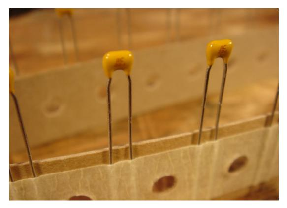
There are two values of ceramic capacitors in WTPA, 0.1uF – there are lots of them – and 20pf, of which you should have 2. The 0.1uFs get used for a lot, most often for power supply filtering (we call it bypassing). The two 20pFs are used to stabilize the crystal oscillator. Neither are polar.
