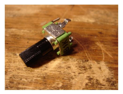
We can see that this pot says B1K (not to be confused with B2K). This means it is a linear taper 1-kilo-ohm potentiometer. The board is labeled for the 500kA ("A" means logarithmic or "audio" taper) and 1kB pots, but the coarse and fine pots are the 10kA and 1kA pots respectively.
