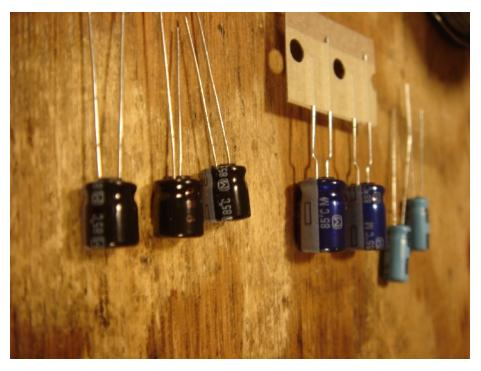
There are three kinds of electrolytic caps: the 470uFs (the big guys), the 22uFs (the black ones) and the 1.0uF (light blue in this photo). The colors aren't important, the numbers are. They'll all be labeled. The big guys are the main power supply filters, the 22uFs are filters for analog references and also the audio output AC coupling, and the 1.0uF caps are inter-stage audio coupling caps.
