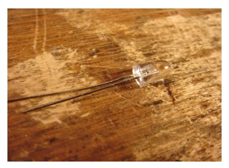
The LONG LEAD on the LED is the anode (positive). It is oriented towards the top of the PCB everywhere in WTPA. There is also a flat on the other side of the LED (the cathode) which matches the diagram on the PCB.
