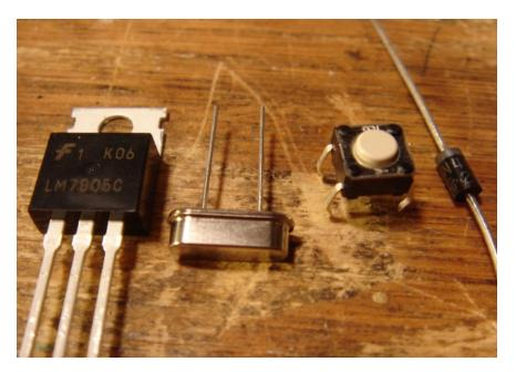
These components are sort of a miscellany. The regulator is really an IC (again) but (again) I took a picture of it because it looks different. The crystal (the silver guy) is what lets the microcontroller generate an accurate clock for it's CPU. The switches are for user input. The diodes (<u>WHICH ARE POLAR</u>) are used to protect WTPA from hooking up power and inputs incorrectly. The bar on one side (the cathode or "negative side") goes in the direction of the arrow on the PCB.
